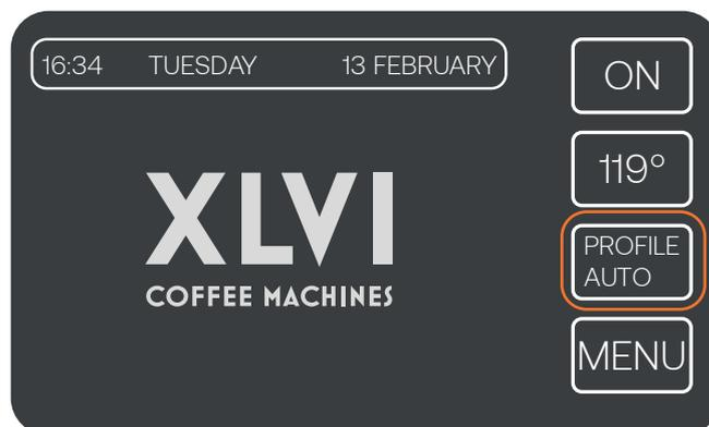
In automatic mode, however, it will be possible to set 4 preset profiles (white, green, red, yellow), being able to vary the TIME, PRESSURE and PAUSE parameters in 5 steps.
